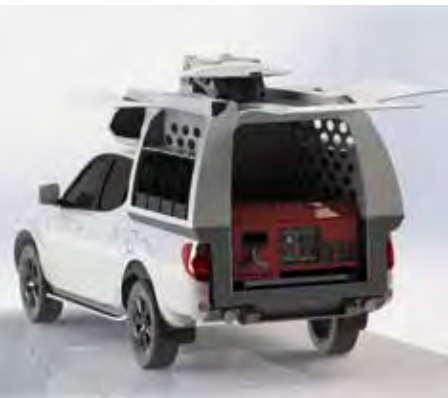
Primetech's family of flexible, demountable MultiPods can be set up for use on a wide variety of different low cost vehicle platforms
