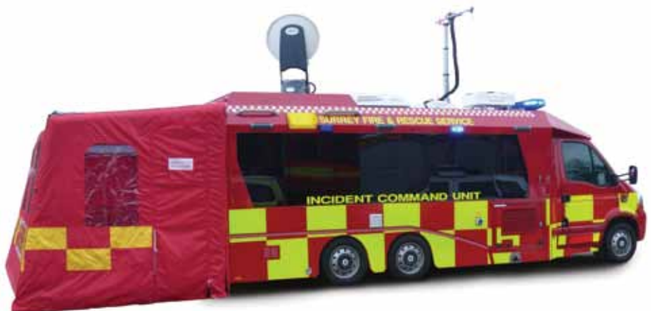
iNetVu Fly-75V antenna. Ka-band satellites transmit up to ten times as much data over the same satellite capacity as Ku-band.
